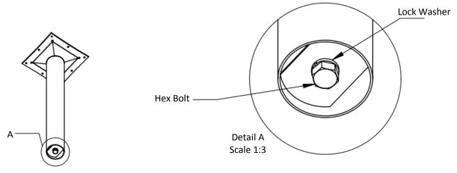
Step 3: Turn the Column upside down. Locate the column around the circular protrusions on the base. Reattach the lock washer and hex bolt.
