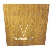
**12-13.** Turn 1/4"T veneer plywood partition so that the "cathedrals" are pointing up. Carefully slide the partition into
