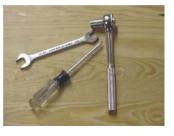
2. Tools needed: 1/2" box wrench and 1/2" socket wrench, and Philips Head Screwdriver.
