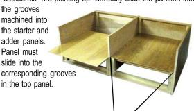
15. Before standing the unit upright, place wood screws as shown in BOTH sections and tighten. Note:
