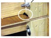
Partition must be pushed all the way <u>into</u> the groove in the underside of the top frame before fastening the partition to the bottom frame.
