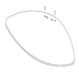
Place the Threaded Posts in the Base inside the corners of the Cover (P4). Secure the Base (P2) to the Inner Support (P3) using two M8 Screws (A). Tighten Screws with Allen Wrench (E).
