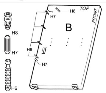
The height of the Top (C) is optional. Select the height that suits your needs. If it wasn't done during assembly of the Base Carrel (LC36), screw three Rafix Bolts (H8) into the appropriate set of predrilled holes in the Side Panel (B) where indicated. These should match the bolts already installed on the Left Side Panel (A) of the Base Carrel (LC36)
