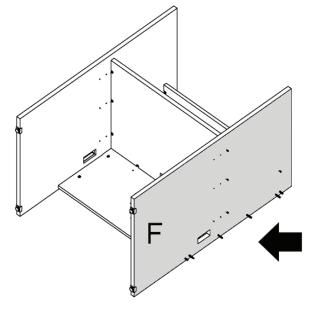
Position the Back (D) as shown onto the bolts and dowels of the Divider (F). Turn the arrows of the cams (H1) clockwise to secure.
