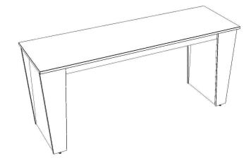
2. Place work surface face down on a protected surface. Position bases on end of table so the inside vertical panels of the bases make contact with the apron rail. Secure with included 1" wood screws
