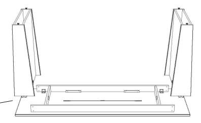
3. Once bases are securely fastened to the work surface use included 1 3/4" wood screws to fasten the the bases to the table apron.
