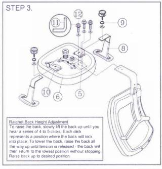
raise and lower the back several times after assembling the chair to insure smooth functioning. MECHANISM INSTRUCTIONS (A) SEAT HEIGHT ADJUSTMENT :
