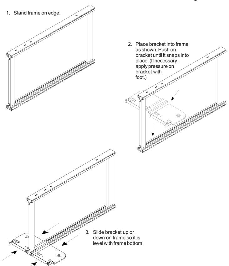
4. If assembling only a single unit, fasten bracket to frame with two 1/4"-20 x 1" hexhead machine bolts. If assembling a range, brackets must not be bolted until entire
