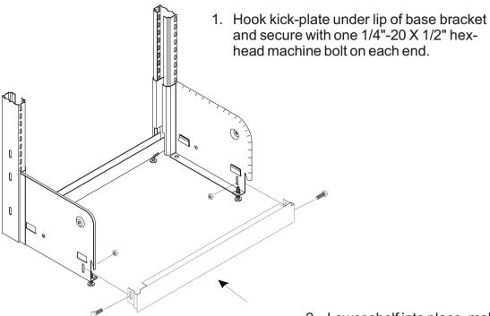
2. Lower shelf into place, making certain that shelf flanges are inserted into the two tabs on each base bracket.
