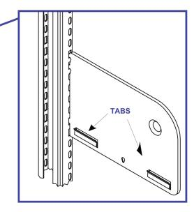
2. Lower shelf onto brackets, making sure that shelf edges fit securely into shelf bracket tabs. Tap shelf firmly into place.
