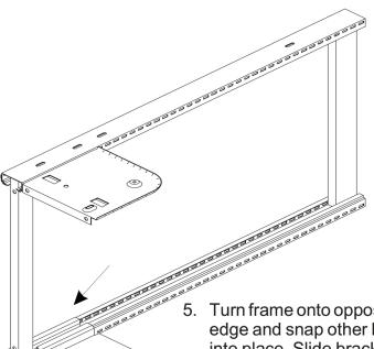
5. Turn frame onto opposite edge and snap other bracket into place. Slide bracket up or down so it is level with frame bottom (as in step 3).
