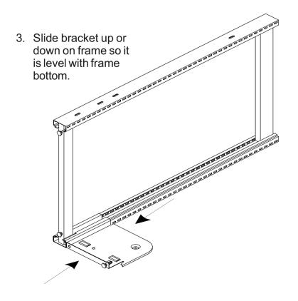
4. If assembling only a single unit, fasten bracket to frame with two 1/4"-20 x 1" hex-
