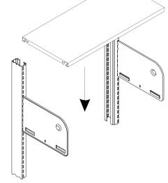
Once assembled, shelf and brackets together may be easily moved up or down on unit as needed.
