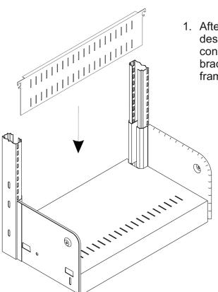
After inserting base shelf as previously described, lower back stop onto unit, connecting the backstop hooks onto base bracket between the base bracket and frame (as shown in inset below).
