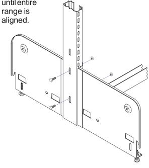
5. Turn frame onto opposite edge and snap other bracket into place. Slide bracket up or down so it is level with frame bottom (as in step 3).
