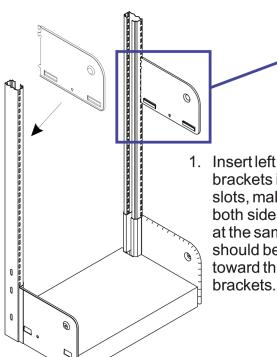
1. Insert left and right shelf brackets into frame slots, making sure that both sides are inserted at the same level. Tabs should be facing in toward the shelf on both brackets.
