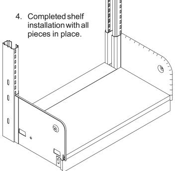
If installing a divider base shelf, see inside back cover for backstop installation instructions
