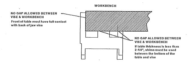
Figure 1: Mount Back Jaw Casting to Work Bench
