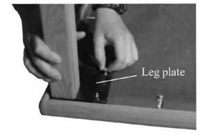
3. Each leg plate will have 3 heavy duty bolts. Each bolt will have 1 lock washer. Place lock washer on bolt as shown. *Check each bolt hole in table top and remove any trash collected during shipping*.
