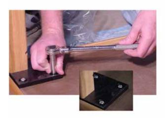
6. Using a 1/2" socket wrench slowly tighten each bolt until the lock washer has "flattened out" but is not "spreading out" from underneath the bolt head. The head of a fully tightened bolt will not rise above the recessed area of the leg plate.
