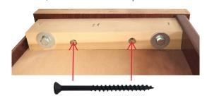
13. Use 2-1/2" long screws to screw through the wood blocks and into the upright panels.
