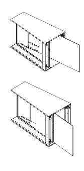
5. GENTLY SLIDE BACKS INTO PANEL GROOVES COMPLETLY INTO THE PANEL UNTIL IT REACHES THE BOTTOM OF THE TOP FRAME CAP.
