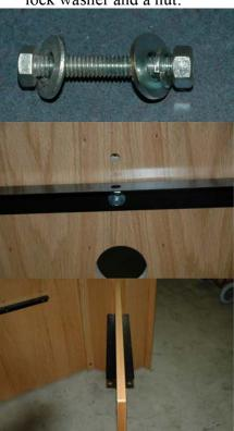
6) Use three 5/8" bronze connector bolts with bronze end caps to close unused holes on the Adder panel:
