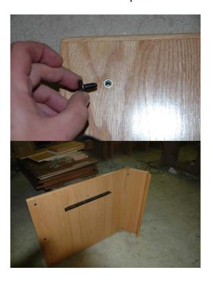
4) Align and attach an Adder panel with the existing back panel and an additional back panel. Attach these three parts with three 2-3/4" bronze connector bolts and bronze end caps, being sure to tighten all connector bolts with an Alan wrench:
