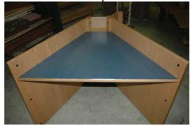
8) Using 1" hex head bolts, each with a washer and lock washer, attach the work surface to the brackets:
