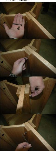
5) Attach two metal brackets to the Adder Panel using three 2-1/4" hex head bolts, two washers, a lock washer and a nut:
