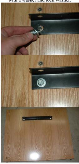
2) Stand the panel up and attach one end to a back panel using three 1-1/4" bronze connector bolts:
